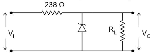
For stable operation of this circuit, the input voltage  $V_i$  must have a range
